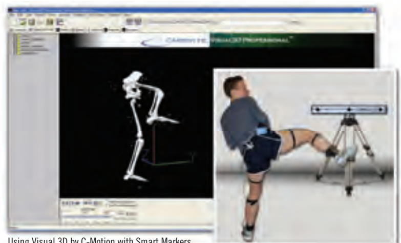
Using Visual 3D by C-Motion with Smart Markers
